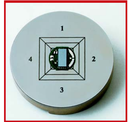
Flip Chip package mounted on fixture
