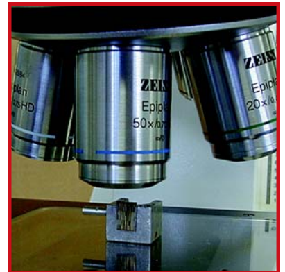
Low profile paddle for microscope viewing
