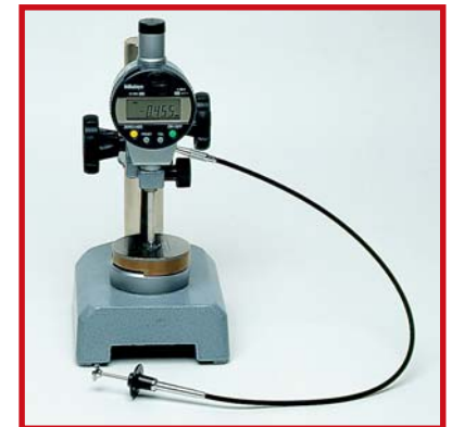
Verify thickness with #120-30010 Digital Measurement System
